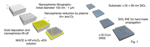
*Fig. 1: Left: fabrication of porous silicon nanowires by nanosphere lithography and Metal Assisted Chemical Etching. Right: fabrication of crystalline nanowires by nanosphere lithography and Cryo DRIE*
